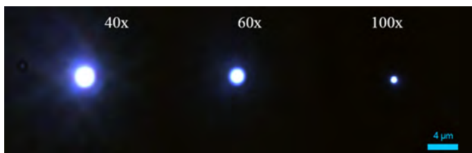
White light spot focusing on specular surface by various objectives.
